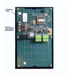
that the driver chip is oriented the correct way.
