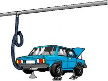
Alentec & Orion AB s swinging arm is a simple and space-saving method to increase the coverage of the exhaust hoses for example in truck workshops and car service halls. The double articulated swinging arm fitted with an exhaust hose enables the connected vehicles to move within a radius of 8-9 meters from the attachment point of the swinging arm. A balancer keeps the hose away from the floor.
