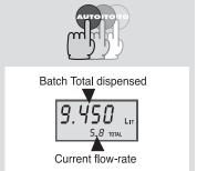
If the flow rate exceeds the range limits, adjust the components of the system (pumps or balancing valves) to comply with them.
