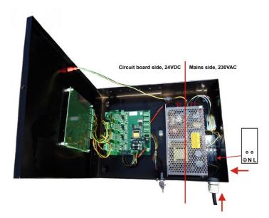
The TSM is equipped with a switched power supply of 150W that can be set for 110VAC/60Hz or 230VAC/50Hz by the internal switch shown by the yellow sticker.
