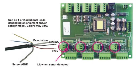
Correct TankType, TCMAddress and TCMPort should be set using with WinDB Manager MASK = ??, TankType = ??1
