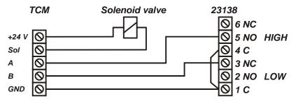
The TCM port should be set to control the appropriate PC tank in relation to the physical tank. Correct TankType, TCMAddress and TCMPort should be set using with WinDB Manager.
