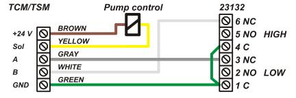
The TCM port should be set to control the appropriate PC tank in relation to the physical tank. Correct TankType, TCMAddress and TCMPort should be set using with WinDB Manager
